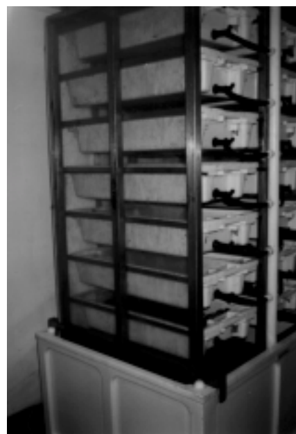
Containers supported on stainless steel frame
