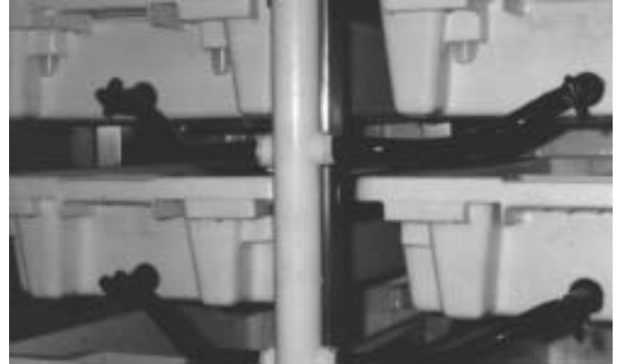
Flexible drain tubes and central drain
