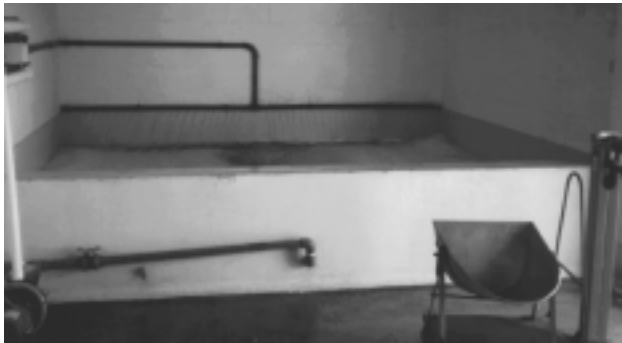
Rectangular shallow tank system
