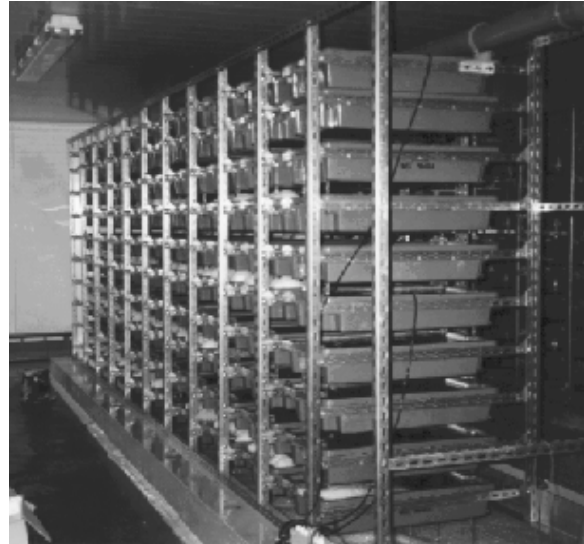
Vertical stack system using Seafish containers
